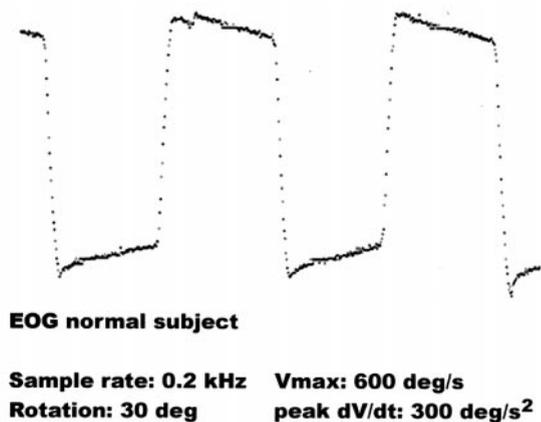
**Figure 5.** (Zacharias) Actual EOG recording digitized from a normal eye and used to apply motion in a similar pattern to the artificial globe to simulate saccadic eye movements.
