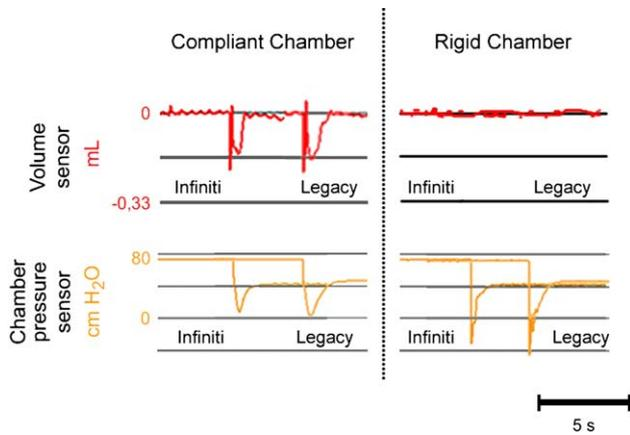
**Figure 9.** Comparison of Alcon Legacy and Infiniti postocclusion surge responses using 500 mm Hg as vacuum limit setting.
