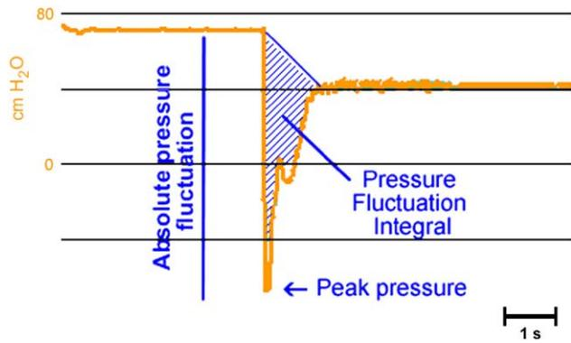
**Figure 8.** Pressure fluctuation characterization during the surge. Pressure fluctuation integral is expressed in  $\text{cm H}_2\text{O} \times \text{seconds}$ .
