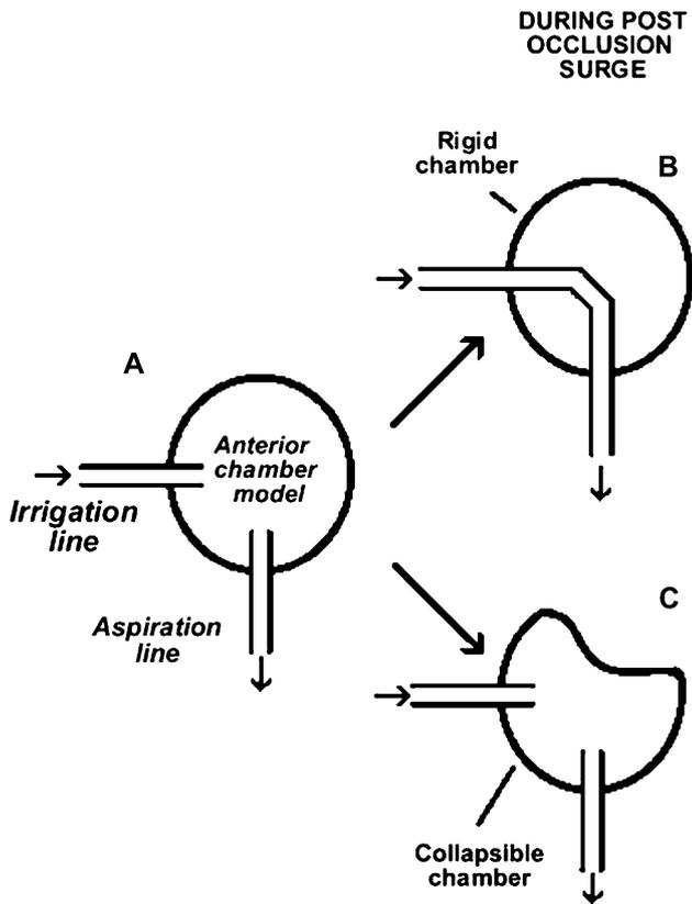
**Figure 10.** Functional models of postocclusion surge (A). A different post-occlusion surge response is observed when a rigid chamber model (B) or a collapsible chamber model (C) is used.
