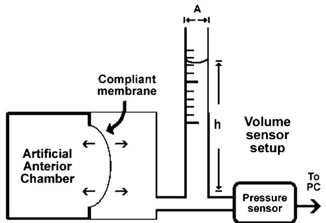
**Figure 3.** Volume sensor array shows a compliant membrane. Measuring the pressure produced by the water column allowed determination of the volume variation inside the collapsible chamber ( $h$  = column height;  $A$  = cross-sectional area).
