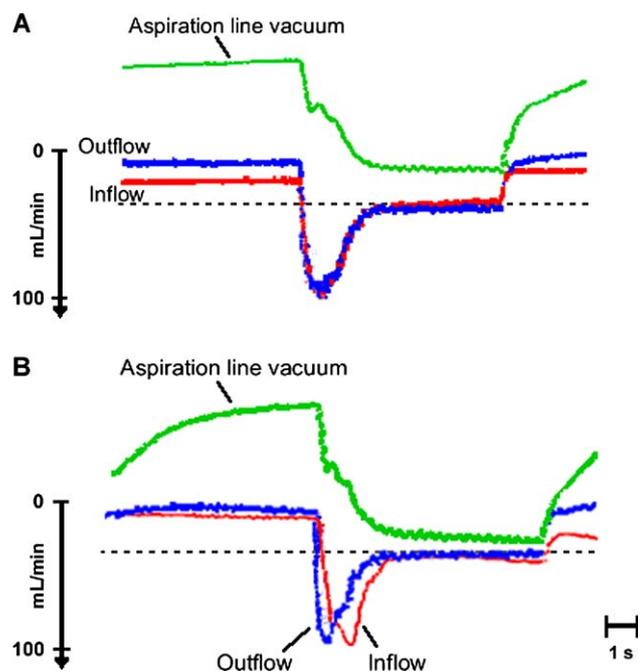
**Figure 6.** Outflow and inflow offset during postocclusion surge in a rigid chamber (A) and in a collapsible chamber (B). In the collapsible chamber, outflow increases before inflow, implying a transient chamber collapse. Dotted line reflects the steady-state flow rate.
