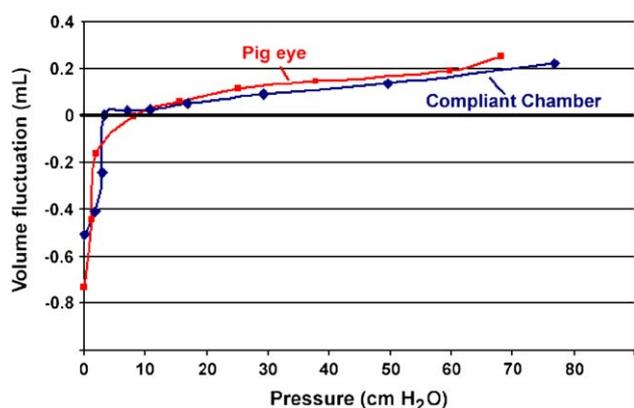
**Figure 4.** Artificial collapsible anterior chamber and pig eye compliance curves. Both show a high compliance in the lower internal pressure range and a relatively small compliance in the upper pressure range connected by an abrupt transition zone.
