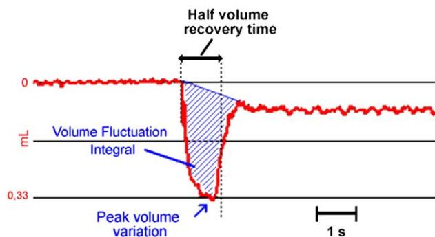
**Figure 7.** Volume fluctuation in a collapsible anterior chamber. Half volume recovery time uses the midpoint between the peak volume variation and the postrecovery volume reading.
