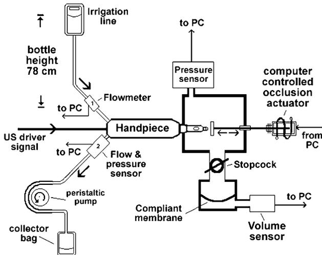
**Figure 1.** Anterior chamber model. A selector valve allows the use of a rigid chamber or a collapsible anterior chamber model. Pressure and volume changes were recorded using a personal computer, which also controlled an occlusion actuator.
