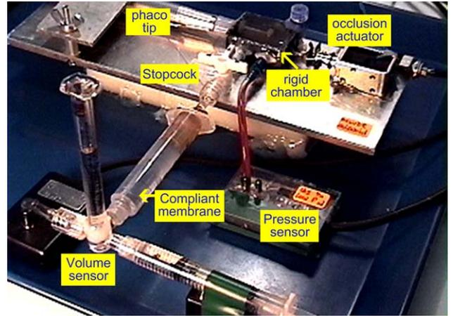
**Figure 2.** Phacoemulsification fluidics laboratory setup.
