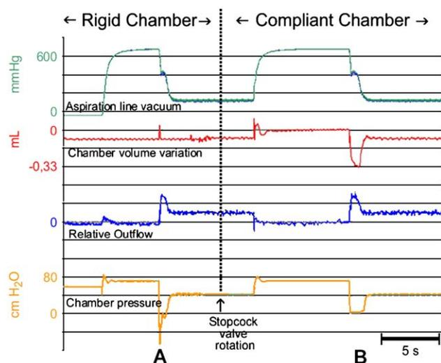
**Figure 5.** Sample of recorded data from an Alcon Infiniti with a vacuum limit setting of 670 mm Hg. Rotation of the selector valve converts the noncompliant chamber (A) into a compliant chamber (B).
